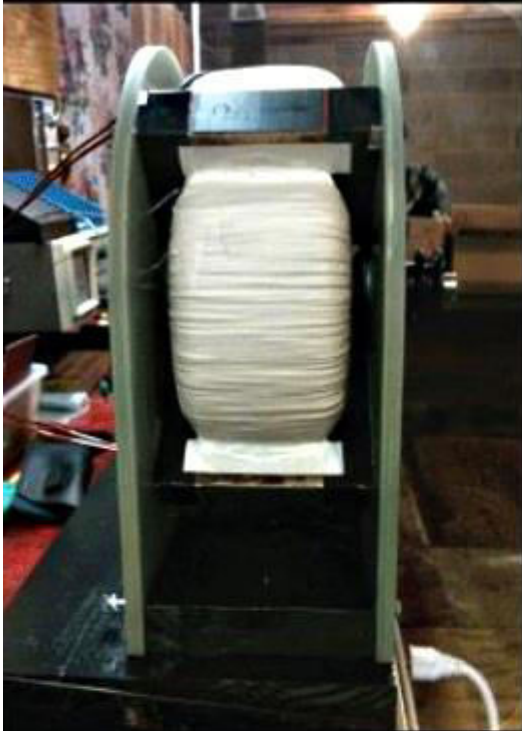
WRAPPED CORE/END PLATES
