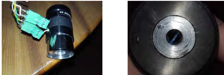
Figure 5 and 6. The detector, a 100 kOhm resistor is in the line of sight /in the focus, the other 3 resistors of the Wheatstone bridge are in the aluminum ring. The ring is placed in a 1.25 inch optical element replacing a Barlow lens
