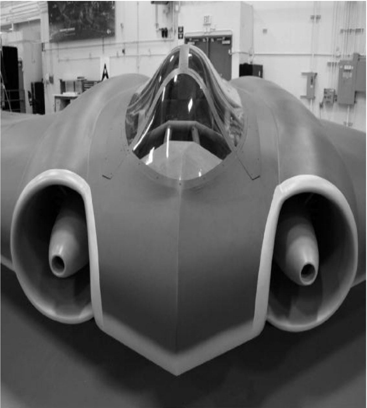
Front of the anti-radar German Horten 229, as reconstructed in the United States by Northrop Grumman.
