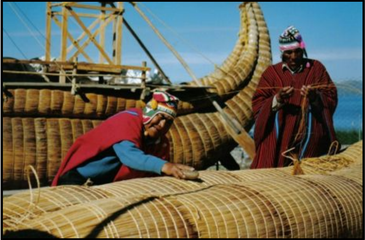
How boats are made using totora reed at Lake Titicaca
